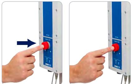
To **disengage** the emergency stop function twist the red button clockwise until it pops out
